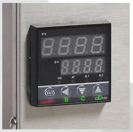
• "B" is Select button, "C" is reduced button, "D" is increase button. how to adjust temperature for 280C. 1st, Turn on heating switch and press "Set" button. 2nd, Press "B" button, when "AT" number light, press "C" or "D" to adjust number for 2. 3rd, Press "B"
